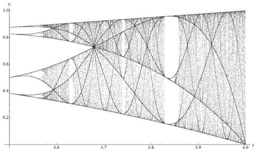
**Figure 7: The Location of the First Ten Images of the Critical Point (Boundaries) are Plotted on the Bifurcation Diagram**
